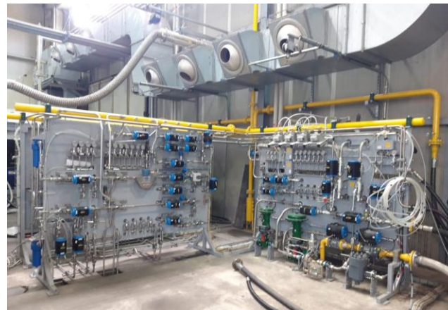
Final load test for each compressor package according to the specific customer working conditions
